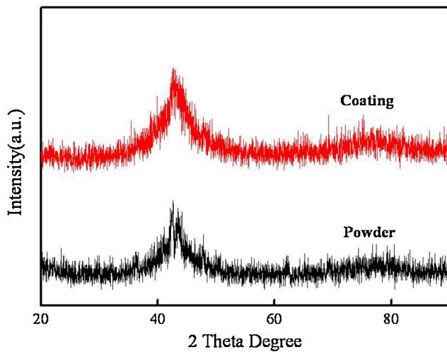
**Fig. 3.** XRD patterns of atomized powders and the as-deposited coating.
