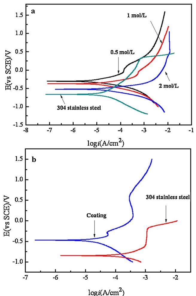
**Fig. 4.** The potentiodynamic polarization curves of the as-deposited coatings in different solution: (a) NaOH solution, and (b) 3.5% NaCl solution.
