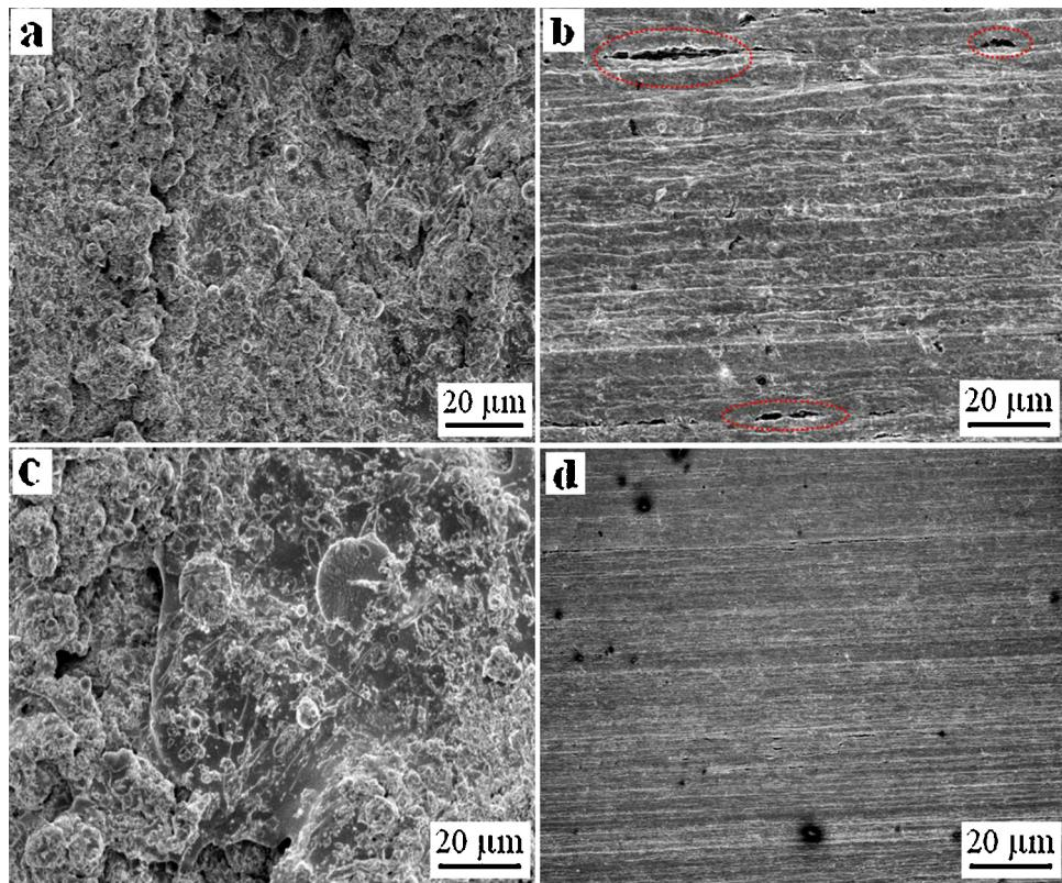
**Fig. 5.** SEM images of the surface after electrochemical test of (a) coating and (b) stainless steel in 2 mol/L NaOH solution, and (c) coating and (d) stainless steel in 3.5% NaCl solution.
