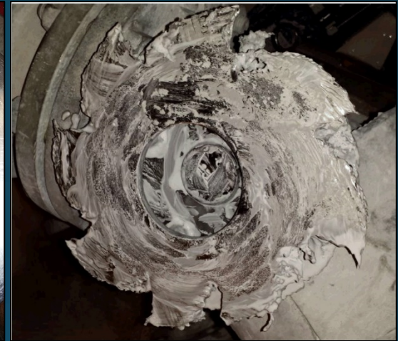
Slurry pump impeller: before and after 3-month service
