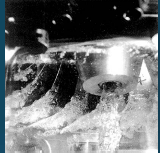
Francis Runner Leading edge, inter blade vortex and traveling bubble
