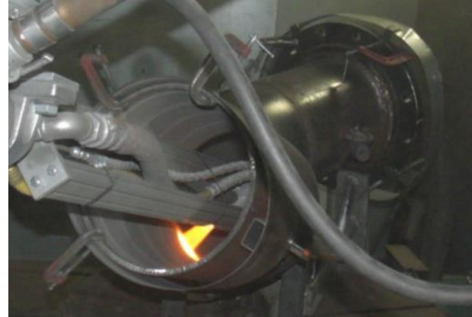
A Double Elbow Sprayed with the Rotating ID Gun
