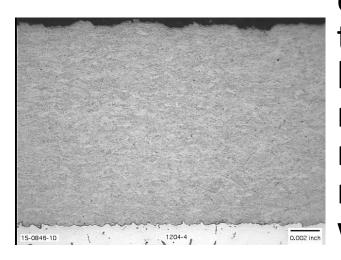
High Velocity Air Fuel (HVAF) – a thermal spray process characterized by a low combustion temperature (<2,010°C | 3,650°F), high particle velocity (800-1,000+m/s | 2,625-3,281 ft./sec.), resulting in low-oxidized, ductile, non-porous, high-bond coatings with high deposition efficiency.
