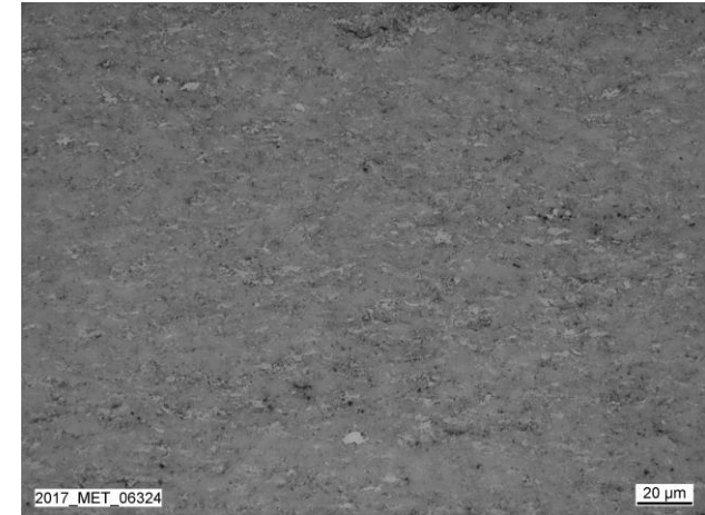
HVAF. Cermet structure with few eta phase
