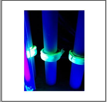
The 50-micron thick coating survives 100 cycles peak loads of +/- 11,000 PSI
